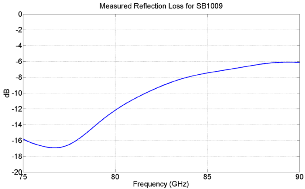
Figure 2 - Measured reflection loss for SB1009 at a 0° angle of incidence.
